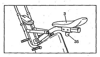
To adjust the position of the Seat (3), first turn the Seat Knob (35) to loosen it. Pull down the Seat Knob, move the Seat to the desired position, and release the Seat Knob. Slide the Seat back and forth slightly until the Seat Knob locks into place. Turn the Seat Knob to tighten it. Push on the Seat to make sure that the Seat Knob is engaged in one of the holes in the underside of the Seat Frame.
